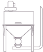
The infeed hopper to a Pneumatic Conveyor system
