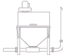
The infeed hopper to a Tubular Drag Conveyor system
